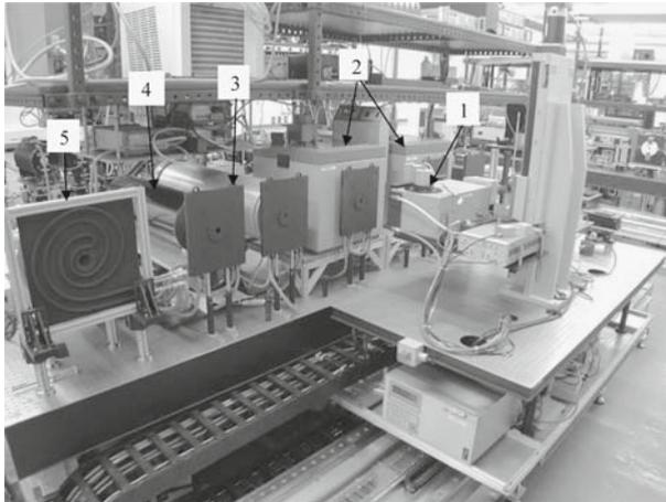
**Fig. 3** Low-temperature cluster of the AIRI Facility: 1—tunable filter comparator, 2—water-bath blackbodies, 3—water heat-pipe blackbody, 4—ammonia heat-pipe blackbody, 5—controlled-background plate
