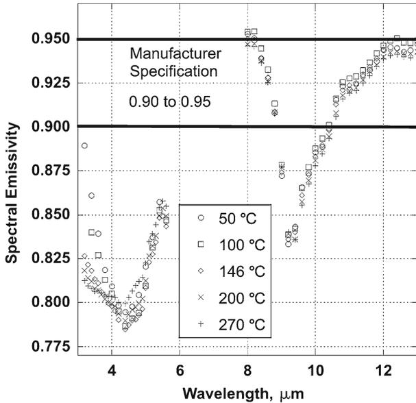
**Fig. 14** Effective spectral directional emissivity of a high-temperature flat-plate BB. Manufacturer specification is 0.95 (+0.00, −0.05)
