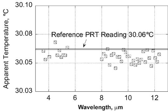
**Fig. 11** Comparison of water HP BB radiance temperature with reference PRT readings. Shown is the difference between measured radiance temperature and contact (PRT) temperature
