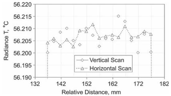
**Fig. 10** Spectrally resolved radiance temperature of the ammonia HP BB, measured relative to the water-bath blackbodies. Reference PRT reading is  $30.06^\circ\text{C}$
