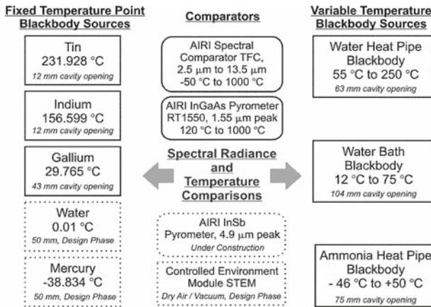
**Fig. 2** Existing (solid boxes) and anticipated (dashed boxes) AIRI components employed in the radiance temperature and spectral radiance scales realization
