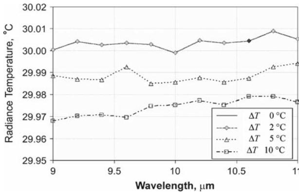
**Fig. 5** Evaluation of spectral comparator uncertainty due to spectral mismatch and detector non-linearity by measuring the same blackbody with variable offset of the reference blackbody temperature. Contact temperature sensor reading of the source under test is 30.08°C
