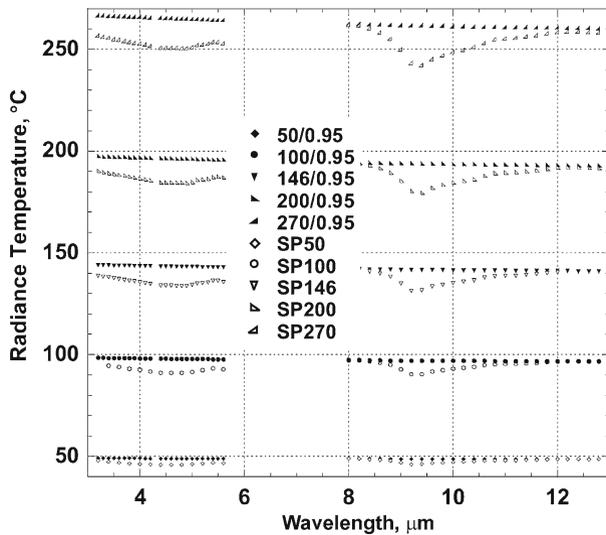
**Fig. 13** Expected and actual radiance temperature of a high-temperature flat-plate blackbody. Light symbols denote anticipated radiance temperature calculated using set-point (SP) temperature, nominal emissivity of 0.95, and background temperature of 24°C. Filled symbols denote measured values
